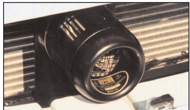
Picture shows the behind the grill mount of a Crown Victoria
